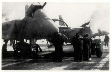
age to an engine. Ice on the ramp is another winter hazard which even the most intensive FOD walk can't prevent. But prior to engine run, it is important to ensure the area around the intakes is free of both ice and snow.
